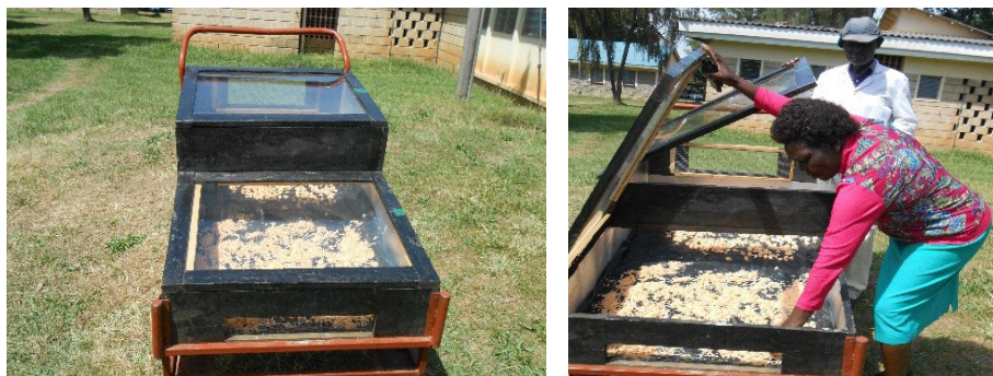
Figure 28: Drying sweet potato chips in a mobile small scale solar drier
