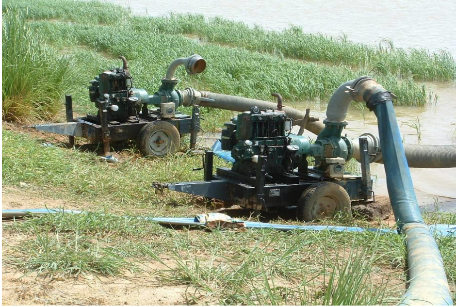
Photo 2: Motor-pump for small scale rice irrigation
