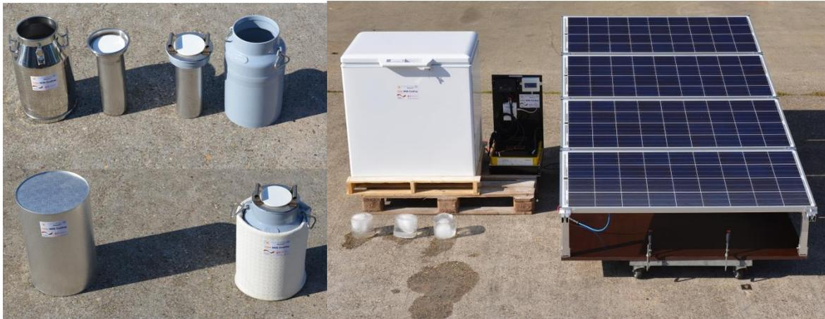
The strategy of milk cooling can be divided into two steps: the production of ice blocks through the use of a smart solar freezer in combination with a control panel that manages the solar energy to efficiently produce ice every day, and the cooling of milk done in the insulated milk cans as shown in Figure 2. The ice blocks produced are placed inside the ice compartment and when the insulated milk can is filled with milk, the ice compartment is placed inside the milk can.
