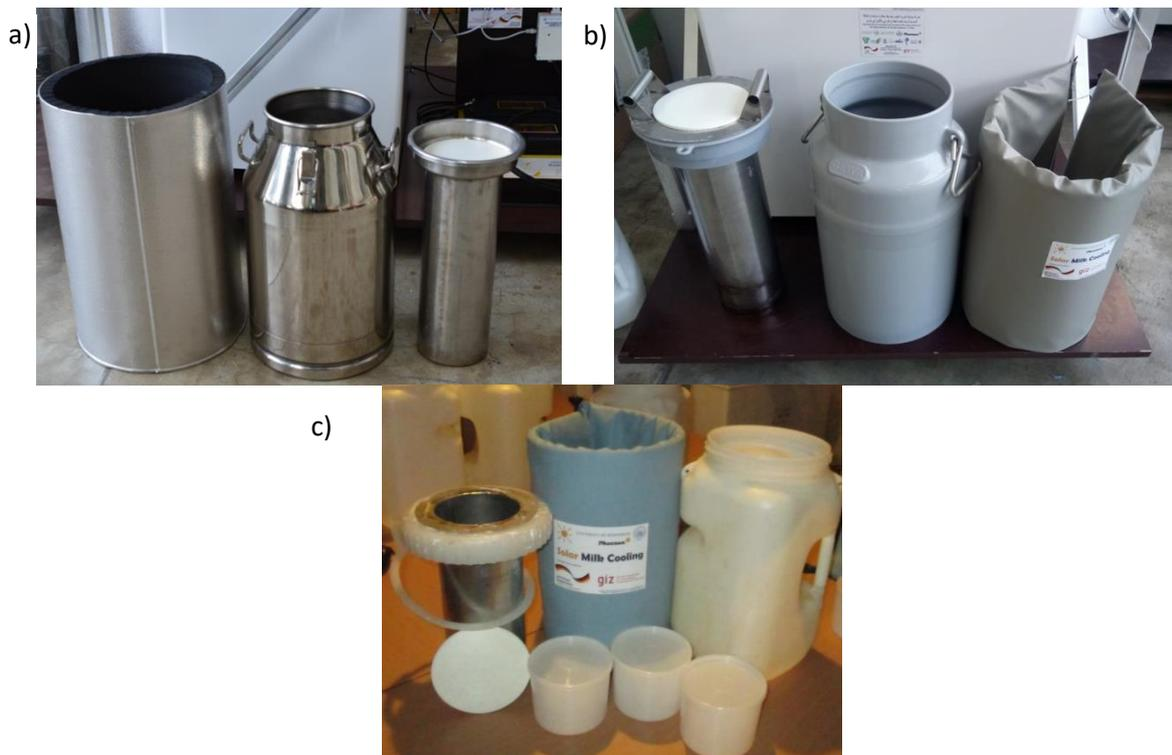
The cooling characteristics of the milk cans shown in Figure 6 were assessed under extreme ambient temperature of 35°C. It was evident that the stainless steel milk can requires a stronger insulation material, compared to the plastic milk can. Nevertheless, the plastic milk cans still required the insulation material in order to reduce the influence of ambient conditions in the cooling process of milk.
