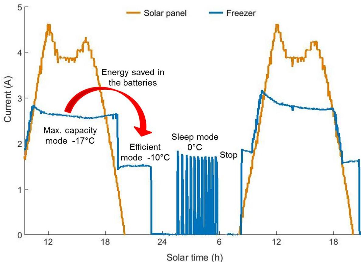
The thermal storage of ice is responsible for the long-term autonomy of the whole ice production and the batteries only help to balance the daily solar energy. Therefore, from the 50kg of ice produced about 16kg of ice can be removed every day according to the evaluation carried out through simulated conditions at the University of Hohenheim (Figure 4). The simulations performed depended on the target country where the system was installed.
