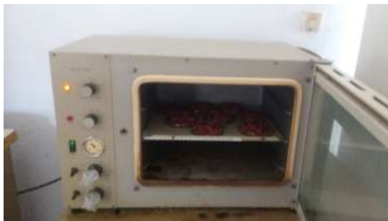
Figure 2: Drying of beans in an oven (Gallenkamp Vacuum oven) for moisture content evaluation.
