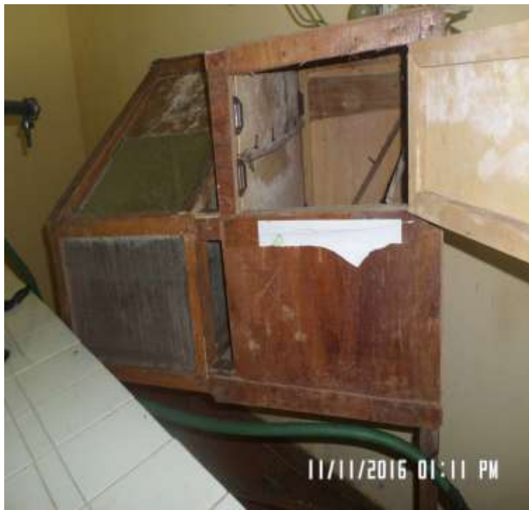
A Fish dryer. For drying fish. It is a wooden cupboard with two chambers- one heated by solar energy and the other by hydro electricity.
