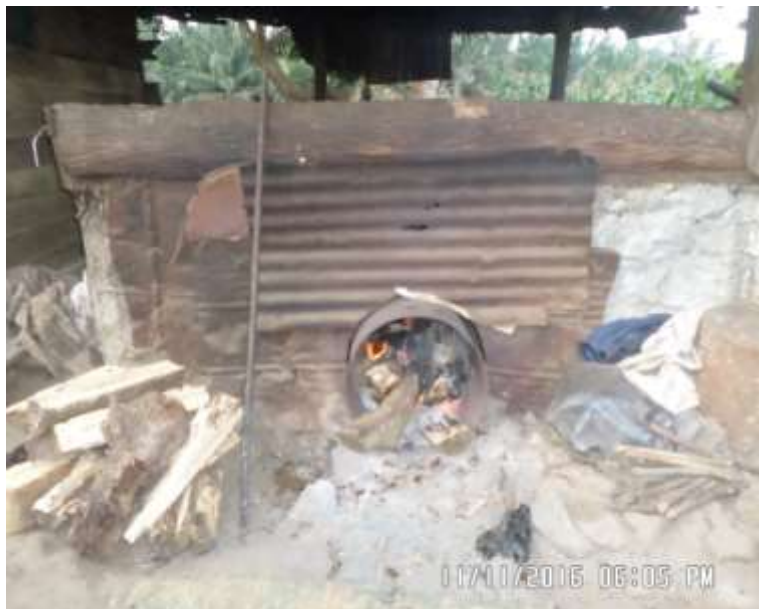
Cocoa oven. It is used for drying cocoa. It consists of concrete walls and a floor of metal rails supporting bamboo bars. It is heated by fuel wood charged in a fire place. The disadvantage is that it wastes wood and therefore not
