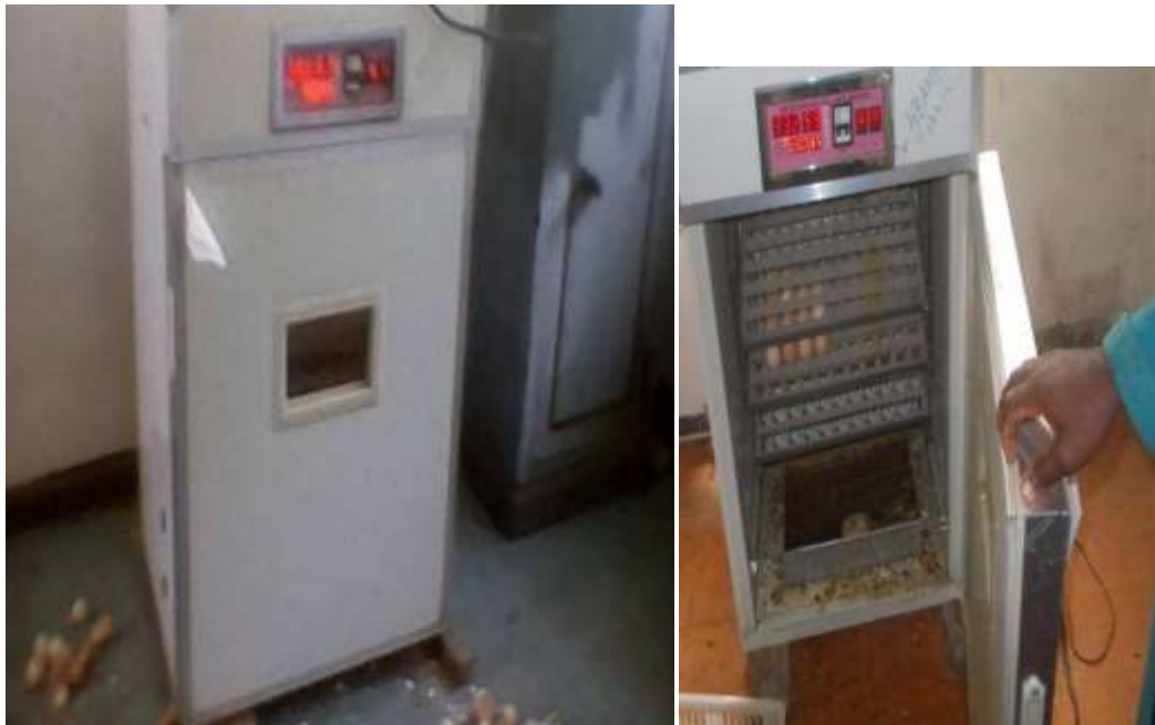
An incubator. For hatching eggs of birds. It has trays containing eggs inserted in for hatching
