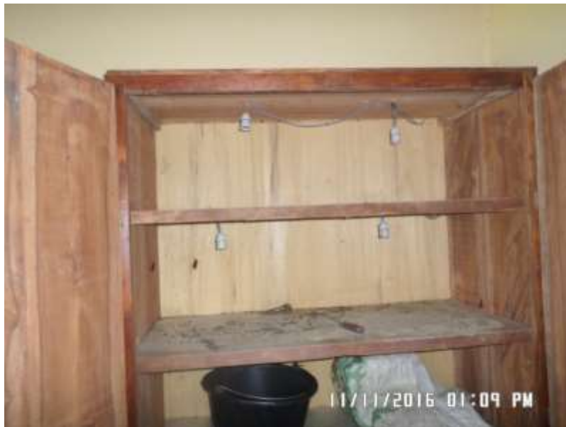
Fish pellet dryer. It is a wooden cupboard with filament bulbs for heating the different compartments.
