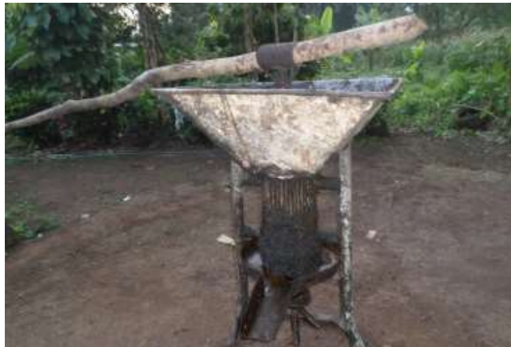
An oil palm hand mill. For processing palm oil. It consists of a pipe and a spiral press in a reservoir mounted on a metal stand. The press is activated by a wooden handle attached at the top of the spring.
