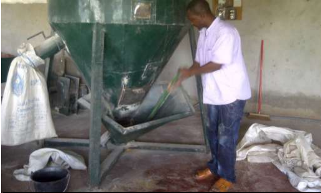
Feed mixer. Mixes different components of animal feed. It consists of a large cylindrical container, a collecting container and an engine and outlets.
