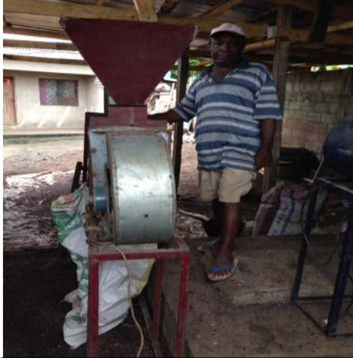
Cocoa "waste" converter: It converts residue from ovens into pure cocoa and separates it from the dirt which is converted into manure (organic fertilizer). It has a blower that separates the dirt from the particles of
