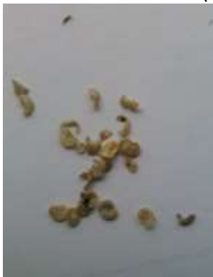
Fig 1. Broken seeds of eggplant by machine
