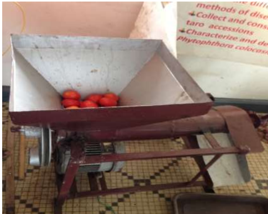
A vegetable seed extractor. Designed and produced by IRAD Ekona (Traditional African vegetable project). It consists of a reservoir a motor mounted on a metal frame. It is used for extracting seeds
