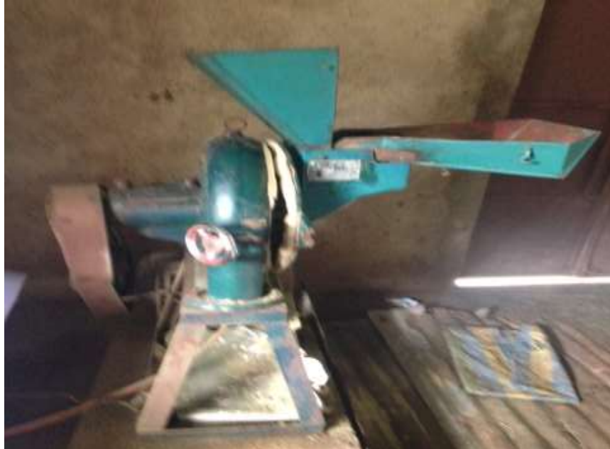
Moringa blender. Used for blending the leaves, roots and seeds of moringa. It has blades in a metal frame and is driven by electricity.
