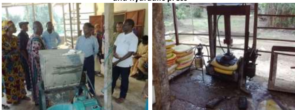
Picture 2: Cassava grating machine powered by electricity (left) and a hydraulic press with bags ready for frying (right)
