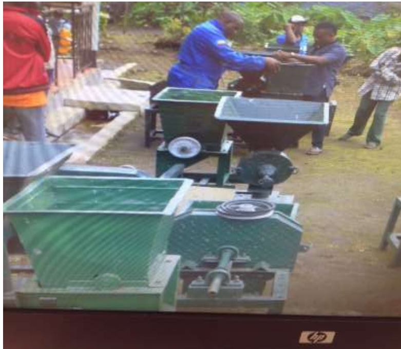
A multipurpose food processing machine. It processes several foods stuff using different properties and parts. It has 3 components ,dry grinder, wet grinder and a grinder for spices. It is powered by thermal energy.
