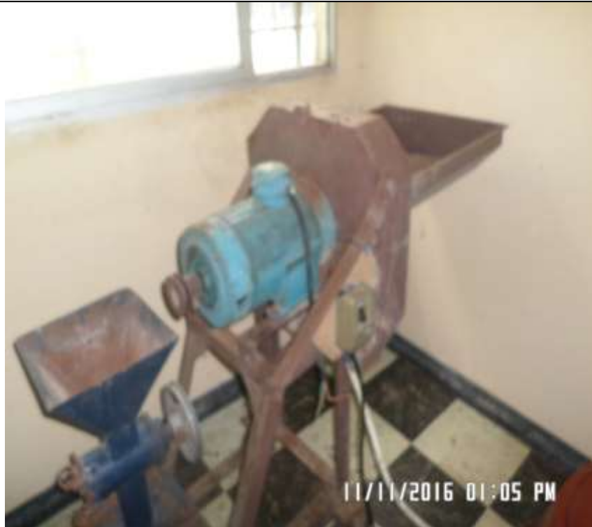
Fish meal Pelleting machine . Used for pelleting fish feed. It has a reservoir, a grinder and a molder.
