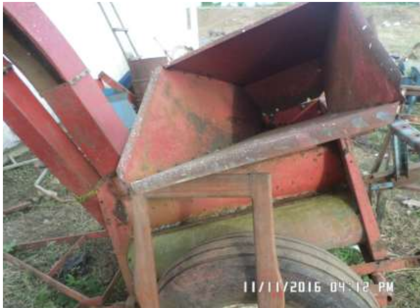
A corn thresher: It is a wheeled hand truck with a rotating arm that removes the seeds.
