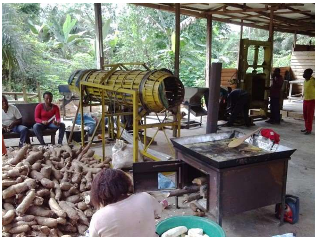
Picture 1: Gari production unit at Besingi showing cassava peeling machine, a gari fryer and hydraulic press
