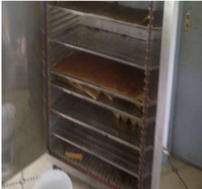
Pellet dryer. Used for drying pellets of animal feed. It is a wooden cupboard heated by electricity.
