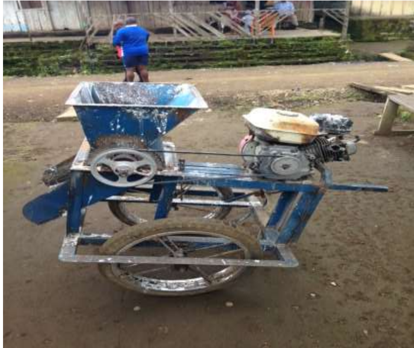
Research results put into use. Grater in use in Tombel Town. It is wheeled and has an engine driven by petrol.
