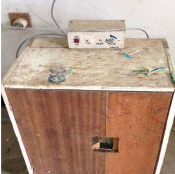
A locally made bird egg incubator. It is a wooden box with an electrically heating component having a thermostat.
