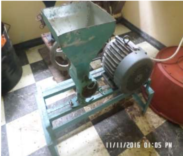
A fish feed mixer. It mixes fish feed for pelleting. It has an engine driven by electricity
